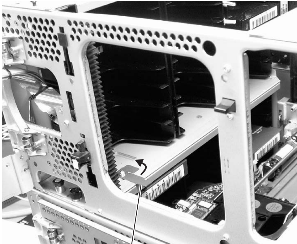
Figure 4-31. Releasing the picker assembly lock mechanism
