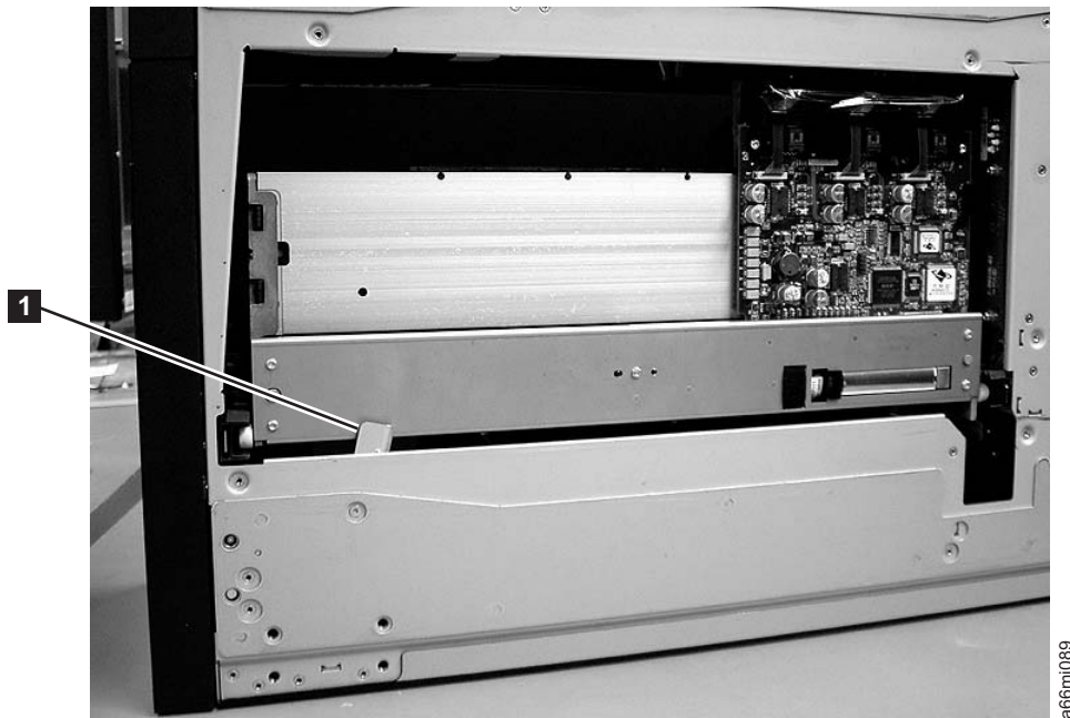
Figure 4-12. Bottom view of picker assembly lock mechanism
