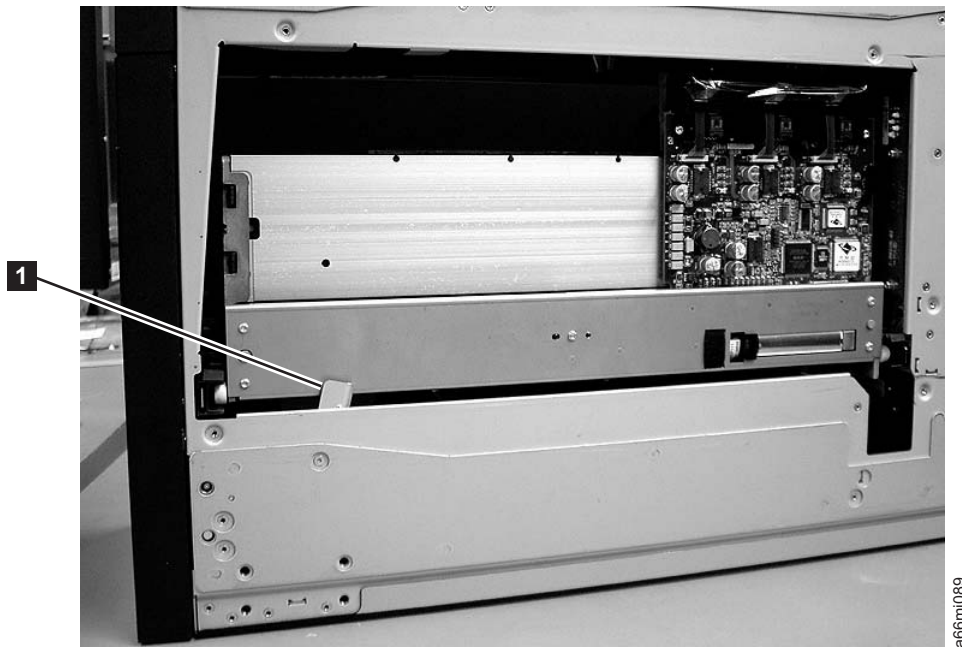
Figure 3-11. Bottom view of picker assembly lock mechanism
