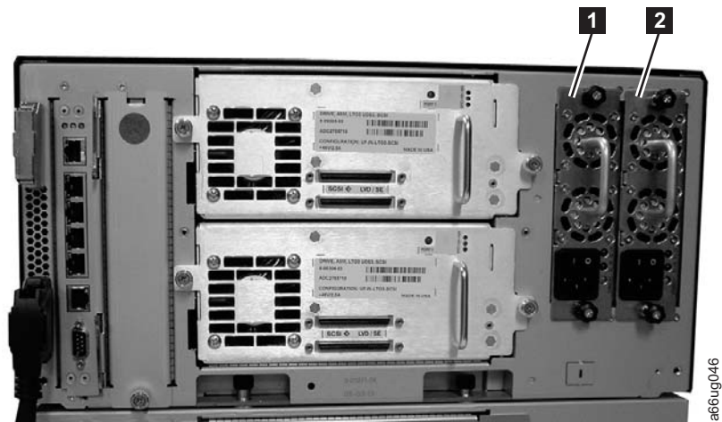
Figure 12-31. Power supplies in a control module
