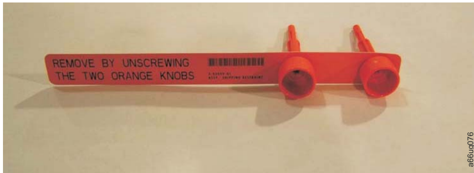
Figure 3-5. M2 picker packaging screws and ribbon removed from the library
