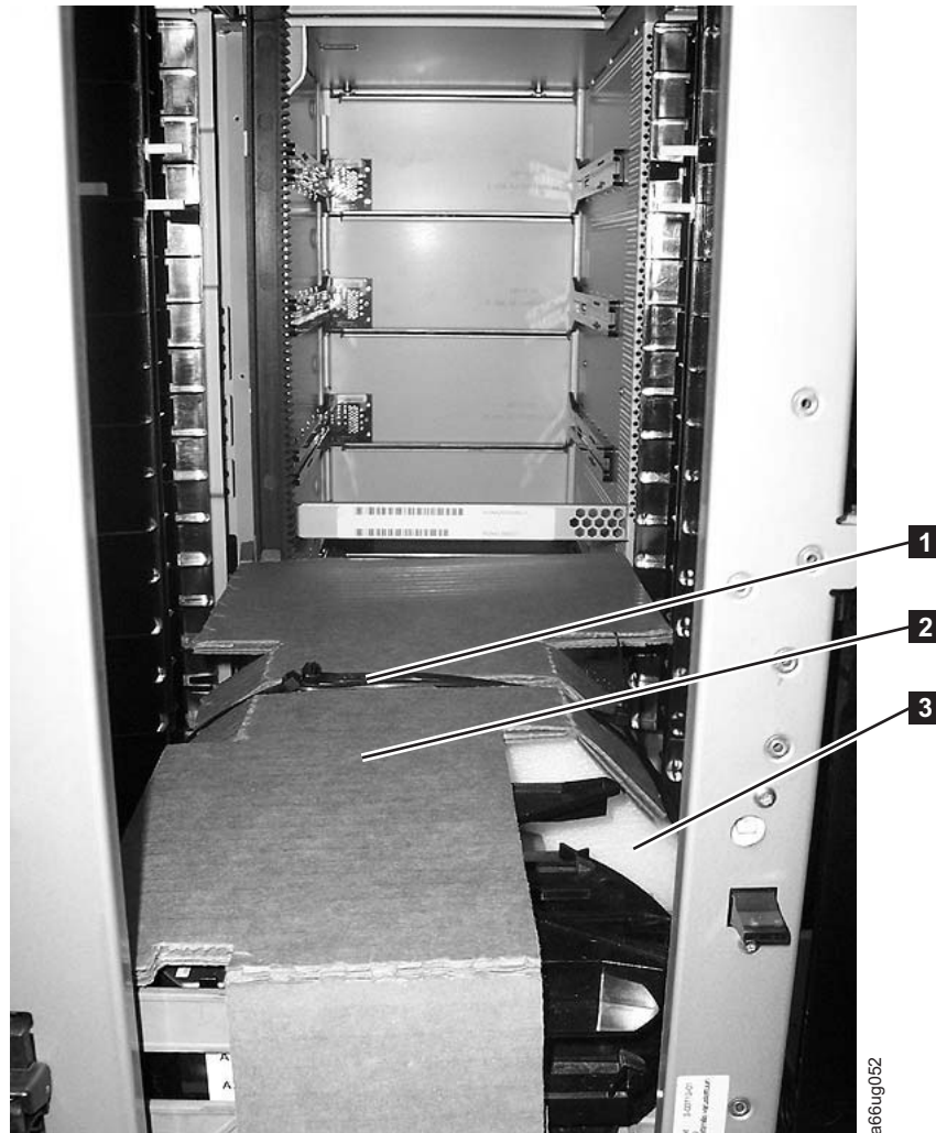
Figure 4-1. Original-style picker with internal packaging material
