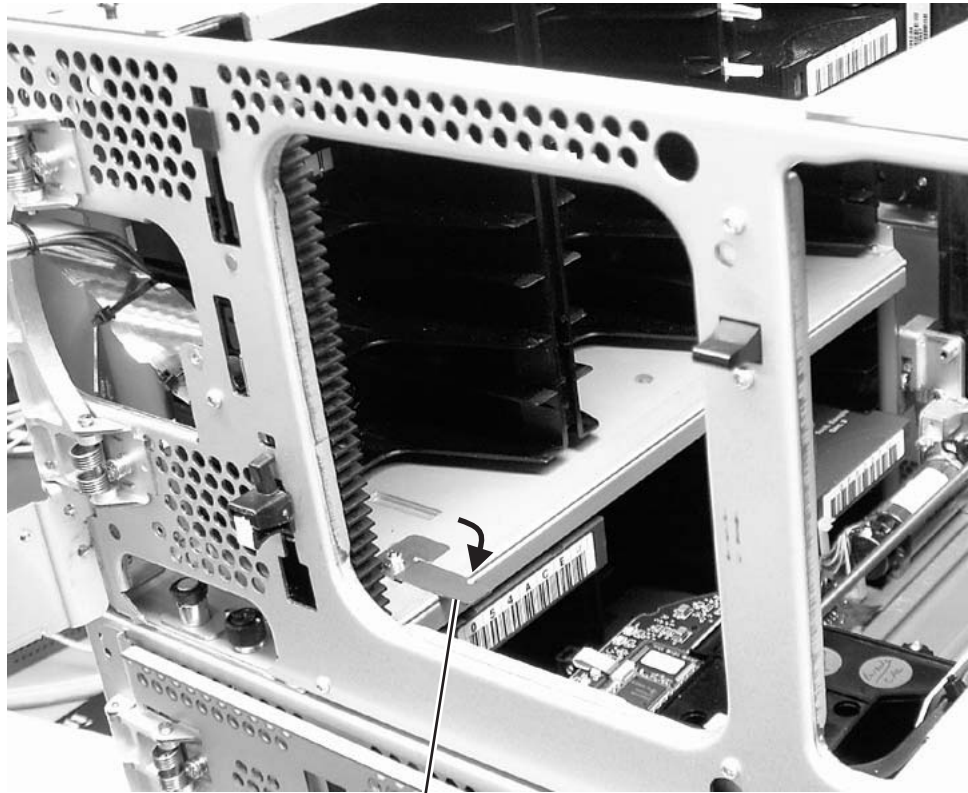
Figure 12-20. Picker assembly locking mechanism
