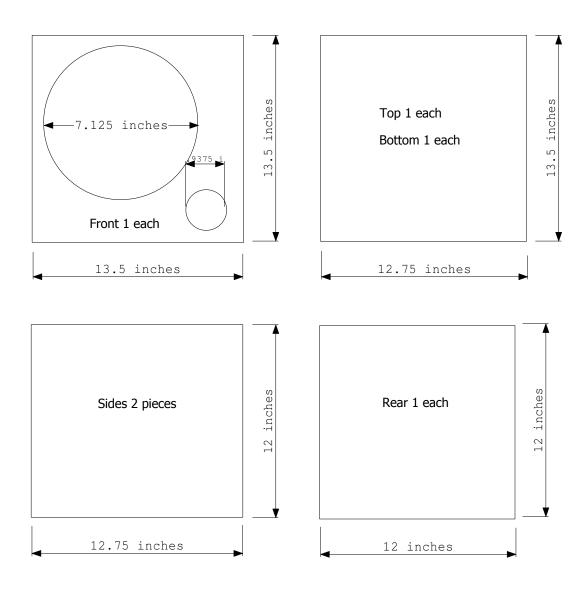
Simple 1 cubic foot sub woofer cabinet. This is designed to work with the Mavin 8" AR sub components.
