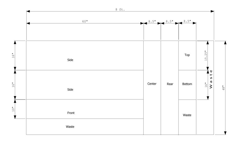
Mavin 6 Pack cutting layout. Each 6 Pack cabinet uses 1 sheet of 4' x 8' material. Use at least 3/4" Plywood, or MDF, or other suitable material. No extra bracing is needed since the interior baffle acts as a brace also. For a pair you will need two sheets of material.
