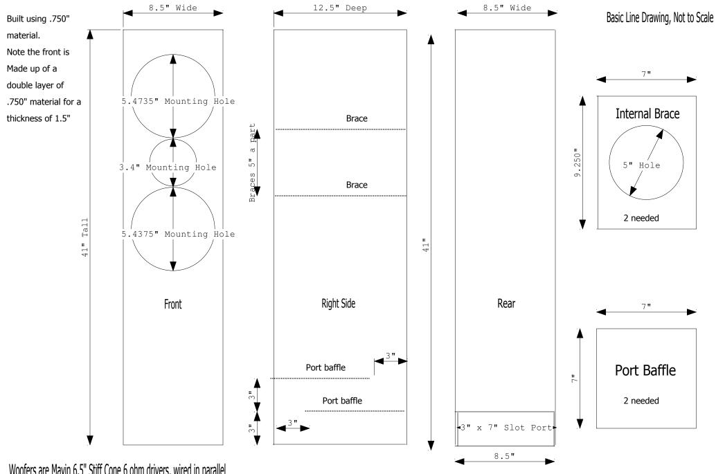
Woofers are Mavin 6.5" Stiff Cone 6 ohm drivers, wired in parallel Cerwin Vega LSE-GF2060 tweeter 4 ohm Using the Mavin 4 ohm 2 way crossover ( 3400 Hz crossover point )
