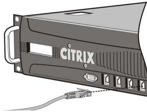
Figure 4 Connecting a Citrix NetScaler Appliance to Your Network
