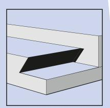
Dovetail slides provide the simplest of all movements. Consists of two precision ground flat surfaces sliding against each other.
