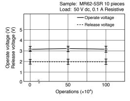
Ambient temperature: Room temperature Driving: 5 V dc, 2 Hz, 50% duty
