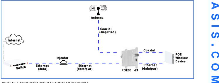
NOTE: RF Coaxial Cables and CAT-5 Cables are not included.
